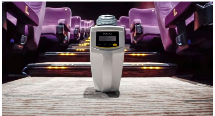
Sartorius' MD8 Air Sampler was set up in a local cinema to capture the air and enable detection of viral particles. (Photo: Sartorius)
